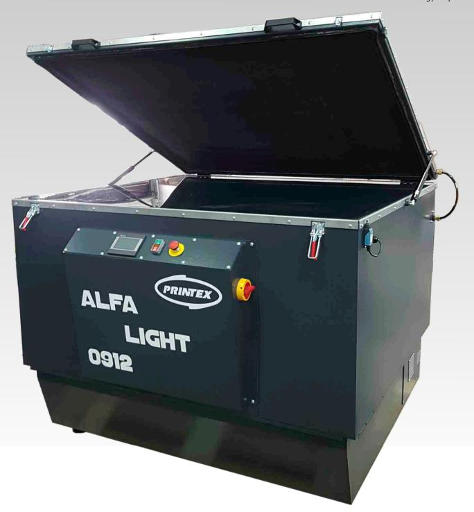
Alfa Light exposure unit comes in 4 sizes:  $70 \times 100$  cm,  $100 \times 125$  cm,  $125 \times 125$  cm and  $125 \times 160$  cm. Standard configuration with vacuum on top gives simplicity of use. Brand name elements used, assure long life for machine
